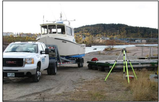
Orion parked adjacent to the RTK DGPS base station prior to launching at a remote survey site on Lake Superior.
