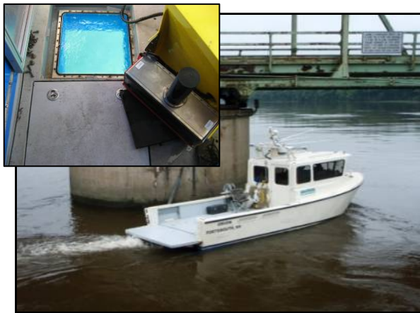
Orion maneuvering around a structural support during a multibeam survey of a bridge on the Kennebec River in Maine. Inset photo shows the Reson 8125 multibeam sonar array just prior to installation of the sonar plug into the moon pool.
